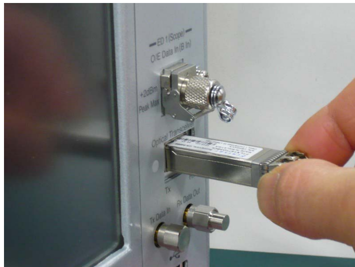
Figure 2.8.1-1 Installing Optical Transceiver
